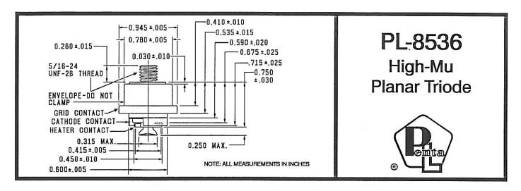
The PL-8536 is a ruggedized, ceramic/metal, high-mu planar triode. It is designed to be used in radio transmitting applications from low frequency to 3 GHz, as a grid pulsed, plate pulsed, or CW oscillator, a frequency multiplier, or as an amplifier.
