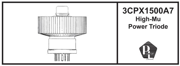
The Penta Laboratories 3CPX1500A7 is a rugged ceramic/metal high-mu power triode, designed with beam-forming cathode and control-grid geometry to allow the simplicity of design and circuit advantages of a triode with the gain of a tetrode.
